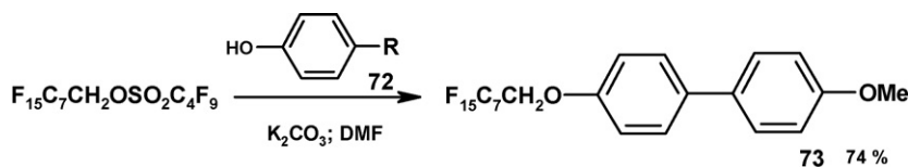
Scheme 26. Preparation of 4'-methoxy-4-(polyfluoroctyloxy)biphenyl.
